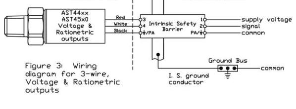
The transducers listed below are designed for installation in EITHER Class I, Division 1, Groups C,D; Class I, Zone 0 Group IIB OR Class I, Division 1, Groups A,B,C,D; Class I, Zone 0 Group IIC hazardous locations when connected to Associated Apparatus as described in note 1.
