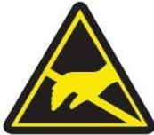
**This product can be damaged by electrostatic discharge (ESD). Handle with appropriate precautions.**
