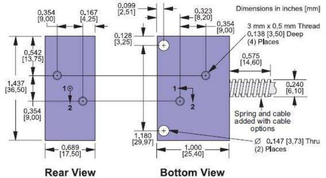
Two through holes and four 3 mm x 0.5 mm threaded holes are provided for mounting.
