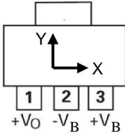
It contains an internal magnet, which provides an auxiliary field of approx. 2.5 kA/m.
