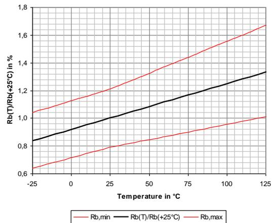
Figure 7: bridge resistance related to room temperature value
