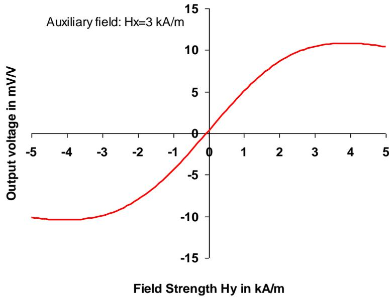
**Figure 4:** Characteristic output curve of KMY 20 S resp. KMZ 20 S for an auxiliary field strength of  $H_x=3$  kA/m
