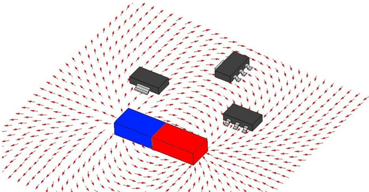
An uniaxial linear magnetic field will generate a linear output within the specified magnetic field range.
