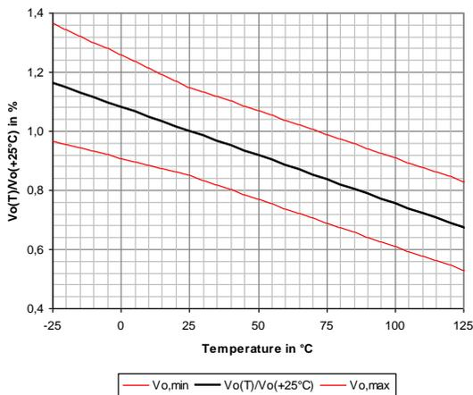
Figure 6: signal amplitude related to room temperature value
