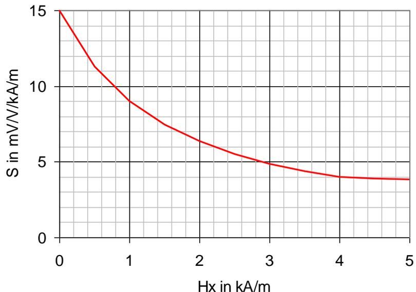
Figure 1: Sensitivity dependence on auxiliary field strength
