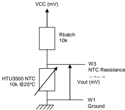
$$V_{OUT} (mV) = \frac{V_{cc}(mV) * NTC_{HTU3500}(\Omega)}{R_{batch}(\Omega) + NTC_{HTU3500}(\Omega)}$$
