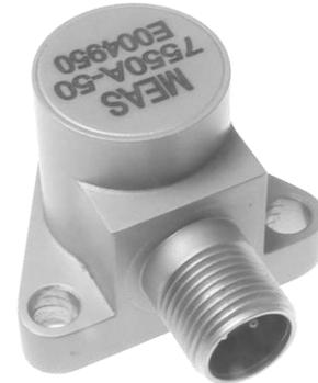
The **Model 7550A** is a high temperature piezoelectric charge mode accelerometer designed for long term health usage monitoring on turbine engines. The accelerometer incorporates an annular shear mode crystal that provides stable thermal response up to +300°C with output sensitivity options of 20pC/g & 50pC/g. The model 7550A is hermetically sealed and features the ARINC three hole mounting configuration.
