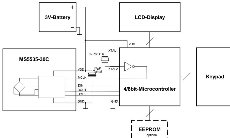
Figure 7: Demonstration of MS5535-30C in a diving computer.
