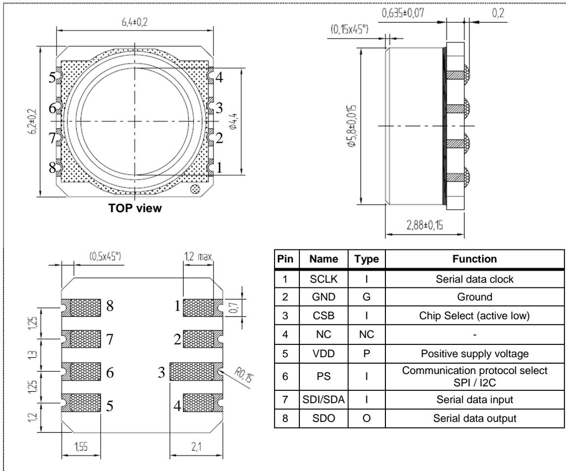
Figure 17: MS5803-05BA package outlines, pin configuration and description
