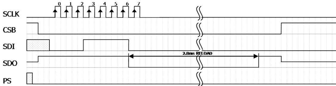
Figure 5: Reset command sequence SPI mode 0
