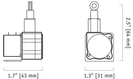
With its ultra compact design the SM1 is the perfect solution when tight space is an issue. At just a little over an inch across, this miniature stringpot offers full stroke measurement ranges from 2½ to 25 inches. A precision plastic hybrid 10K-ohm potentiometer delivers a precise voltage divider output signal that is linearly proportional to the travel of the spring-loaded measuring cable.
