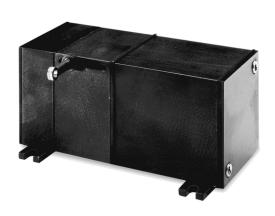
The PT5DN, using a high cycle plastic-hybrid potentiometer, communicates via DeviceNET protocol with programmable controllers in factories and harsh environments requiring linear position measurements in ranges up to 250".
