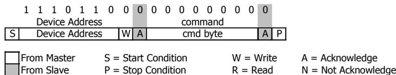
Figure 9: I<sup>2</sup>C ADC read sequence
