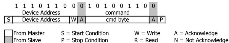
Figure 6: I<sup>2</sup>C Command to read memory address= 011
