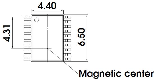
**Figure 7:** Package drawing (Magnetic center)
