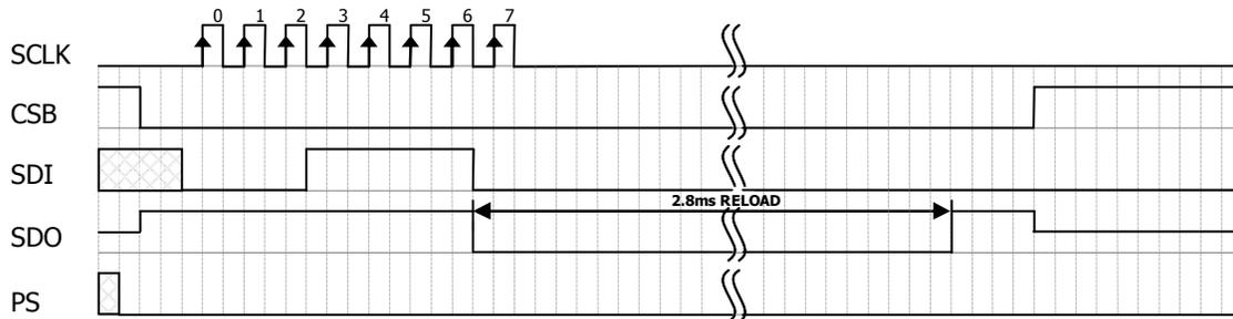
Figure 4: Reset command sequence SPI mode 0
