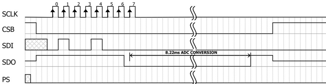
Figure 6: Conversion out sequence, Typ=d1, OSR = 4096
