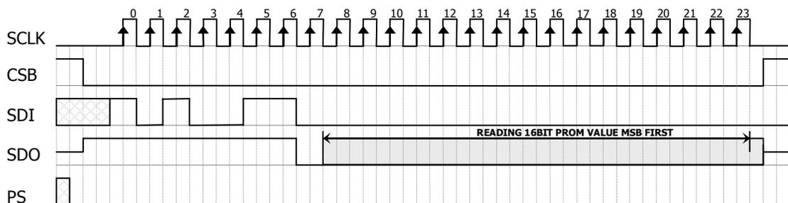
Figure 8: PROM Read sequence, address = 011 (Coefficient 3).
