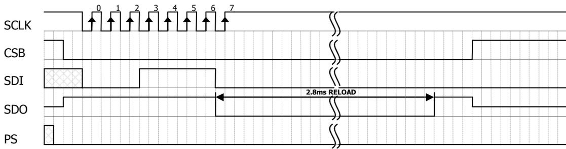
Figure 5: Reset command sequence SPI mode 3
