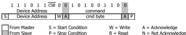
Figure 10: I<sup>2</sup>C Command to read memory address= 011 (Coefficient 3)
