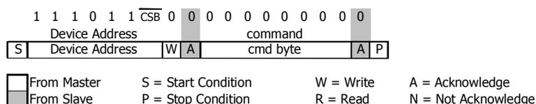
Figure 13: I<sup>2</sup>C ADC read sequence
