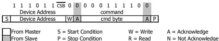
Figure 9: I<sup>2</sup>C Reset Command
