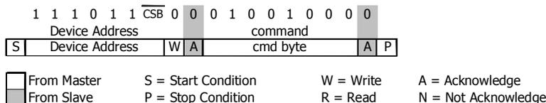
Figure 12: I<sup>2</sup>C Command to initiate a pressure conversion (OSR=4096, typ=D1)
