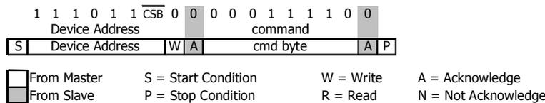
Figure 10: I<sup>2</sup>C Reset Command
