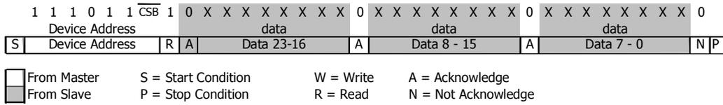
Figure 15: I<sup>2</sup>C pressure response (D1) on 24 bit from MS5803-01BA
