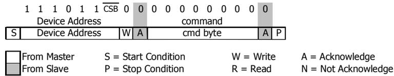
Figure 14: I<sup>2</sup>C ADC read sequence
