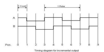
Channel A leads when Channel B shaft is rotated in Clockwise direction.
