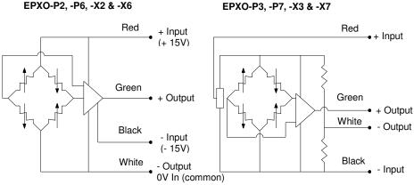
It is recommended that "0V COMMON" of the power supply be grounded if consistent whit proper operation of the instrumentation system.
